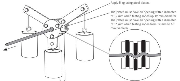
The rope test sample must be 2250 mm long. Separate the inserted plates with spacers at an angle of 120° and apply loads of 5 kg. The rope sample must be pulled through the test apparatus five times. Sheath slippage for type A ropes may not exceed 1 %. Sheath slippage for type B ropes may not exceed 1.5 %.
