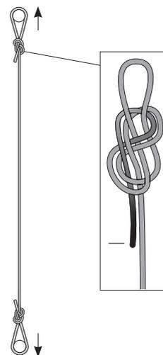
The low stretch kernmantel rope, including terminations with a figure-of-eight-knot, must be able to withstand a force of 15 kN for type A ropes and 12 kN for type B ropes, each for a period of 3 minutes.
