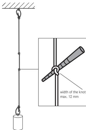
Two single overhand knots are applied to the 3000 mm rope sample with the knot loops running in opposite directions. One end of the rope sample is attached to a suitable fixture. An impact-free load of 10 kg is applied to this piece of the rope for 60 seconds. A test cone is pushed in the eye of the knot. The maximum width of the knots eye must not exceed 12mm.
