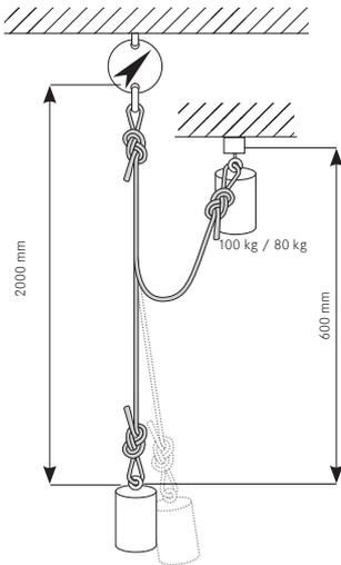
A 100 kg mass is suspended for type A ropes, or a 80 kg mass for type B ropes from the rigid structural anchorage point, by connecting the sample between them for 60 seconds.
