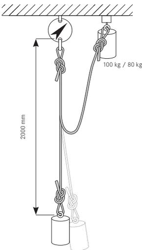
A 100 kg mass for type A ropes is suspended, or a 80 kg mass for type B ropes, from the anchorage point.
