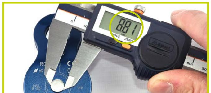
The rivet head has a diameter **larger or equal to 8.7 mm**: the pulley can still be used.
