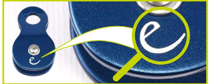
The pulley has a white “e” symbol on the back. The pulley has already been inspected and can still be used.
