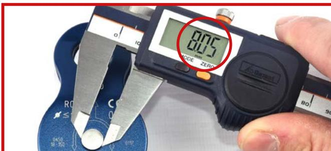
The rivet head has a diameter **smaller than 8.7 mm**: cease to use the pulley immediately and send it to EDELRID for a free replacement.
